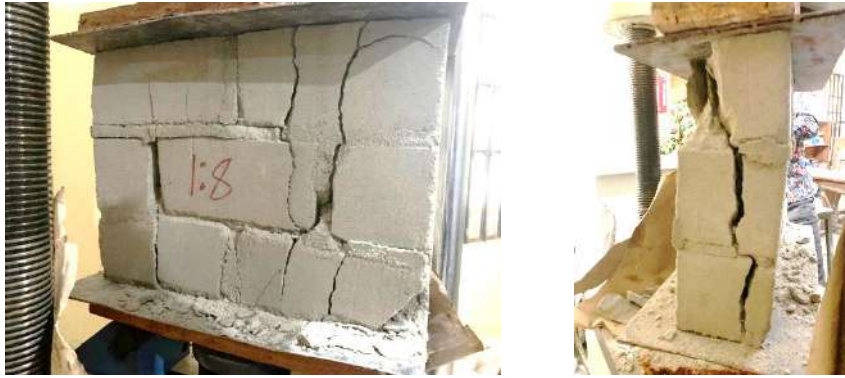
Figure 5. Failure pattern of concrete block prism with 1.975 MPa average mortar compressive strength
