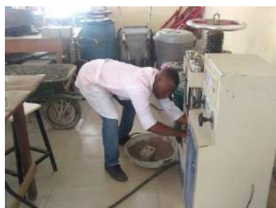
Figure 3. Crushing of Concrete Cubes
