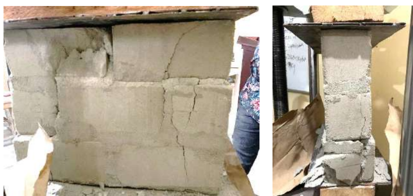
Figure 4. Failure pattern of concrete block prism with 3.979 MPa average mortar compressive strength
