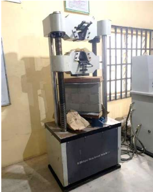
Figure 2. Test setup adopted for uniaxial compressive strength test of concrete block prisms.
